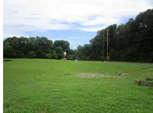
A rain garden can be created in the depressed turfgrass area next to the main entrance. This system can be installed by connecting to the culvert to provide aesthetic value and create wildlife habitat while managing stormwater runoff. A preliminary soil assessment suggests that more soil testing would be required before determining the soil's suitability for green infrastructure.
