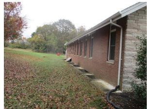
Rain gardens can be installed near the corners of the building to capture, treat, and infiltrate stormwater runoff from the roof. A preliminary soil assessment suggests that the soils have suitable drainage characteristics for green infrastructure.
